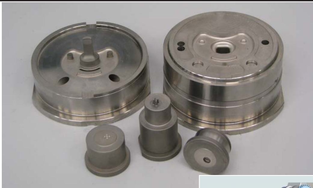
These silicone prototype inserts fit a representative production mold base, allowing exact production simulation.
